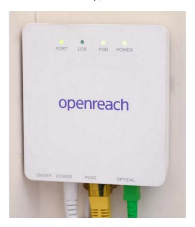
The yellow plug shown in the image above is the RJ45 cable which goes to your router and MUST be plugged into the WAN socket if you already have a suitable router fitted and the ADSL socket which was previous used will no longer be needed.
